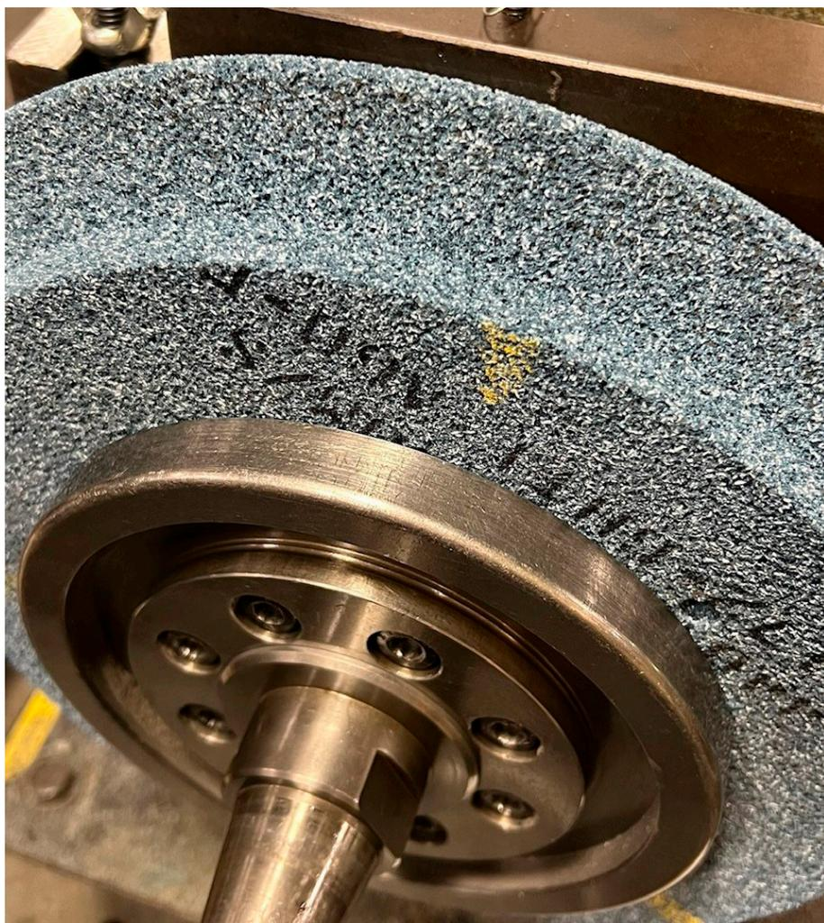
An open porosity, vitrified bonded wheel uses either aluminum oxide grains or high-performance ceramic grains. For profile grinding, it's preferred to use a wheel with induced porosity, or very large pores, to reduce the risk of damaging or scrapping the part. This image shows an open porosity wheel after grinding with no sign of loading.
